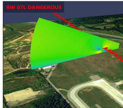
Alert messages are being generated considering the degree of the wake vortex danger for aircraft of various weight categories.
