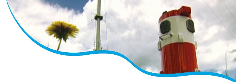
WINDEX-300 is a LIDAR wind profiler providing measurement of horizontal wind speed and direction, as well as vertical wind speed component, at given altitudes with arbitrary assigned increment step.
